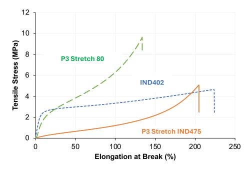
A stress-strain curve of Loctite 3D IND402 and P3 Stretch IND475 show their difference in physical behavior.
