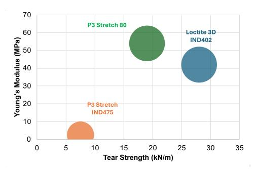
Higher Young's Modulus values indicate that the material is stiffer and has a higher Shore Hardness value. Elastomers with higher stiffness are generally more resistant to tearing.
